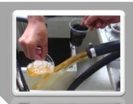
Crystal clear oil after the filtering process The high-precision filtration can meet the standard NAS 7/8 or 3-5  $\mu m$  oil is clear and transparent, invisible impurities. Protect the machine without oil pollution, but ensure the precision of the tools and oil
