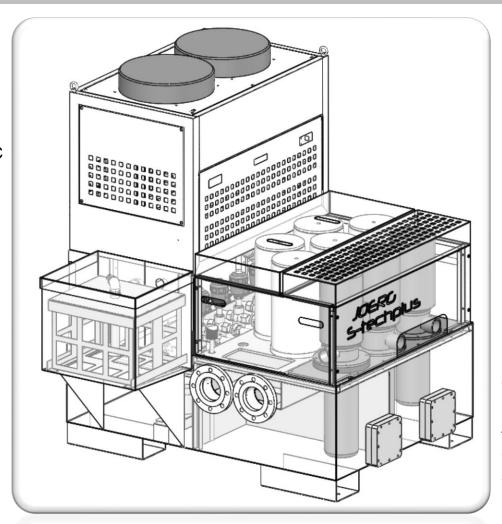
3-5 filter towers with a Filtering grade of 3 µm - 5 µm
